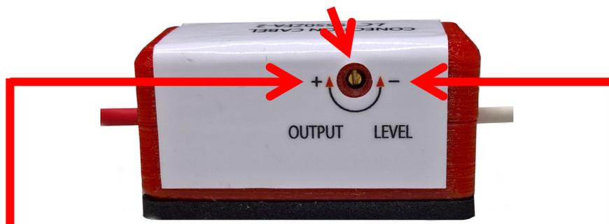
Smaller level adjustments are possible with the externally accessible trim control.
